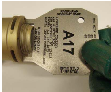
Picture 6C – Use of Stick-Out Gage on the Gas Turbine side of the Flange Joint
