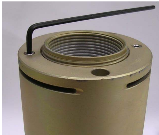
Picture 6 - Loosening of a nut's set screws
