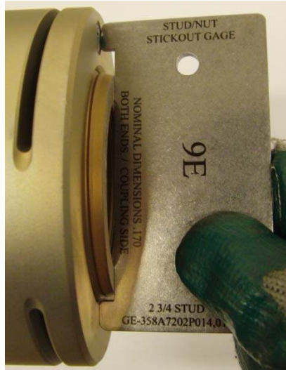
Picture 6C – Use of Stick-Out Gage
