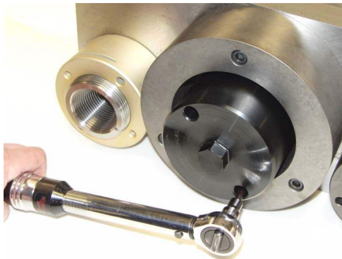
Figure 11G – Tighten screws on stud removal tool
