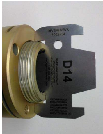
Figure 6A – Use of gage to measure stick-out
