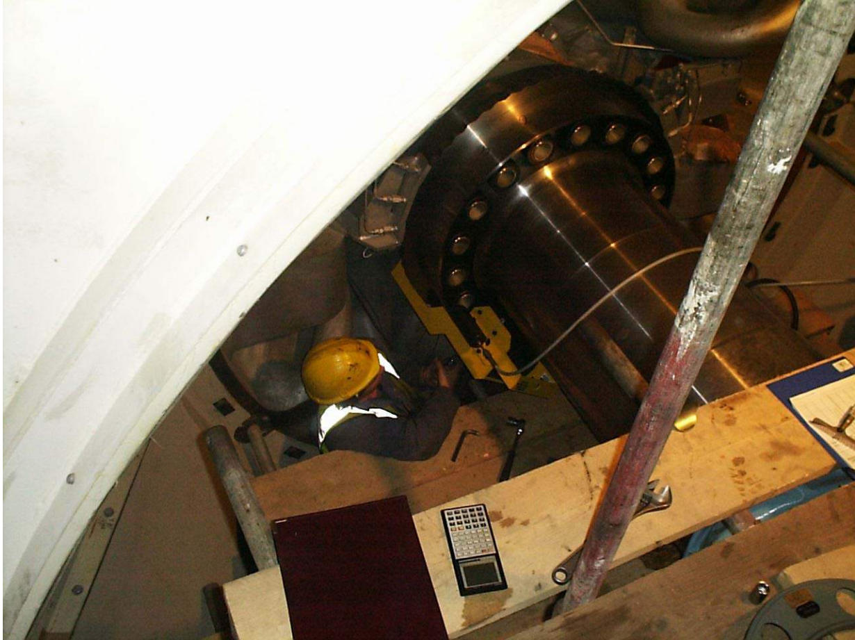
Photo 4 Tensioner in operation while mounted on 9FA turbine
