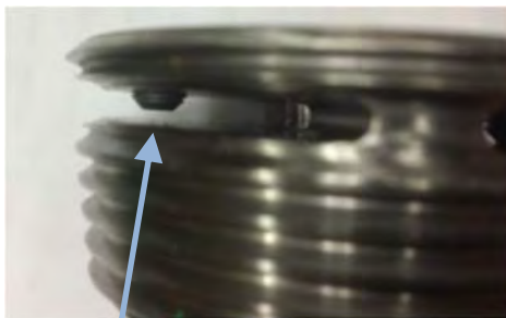
Partially Loose Set screw
