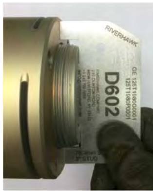
Picture 6F – Use of D602 Stick-Out Gage on HPIP-LP Flange
