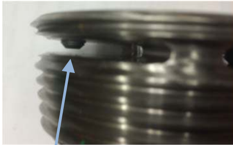
Partially Loose Set screw
