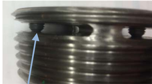
Pressed against Opposite Surface. No Gap
