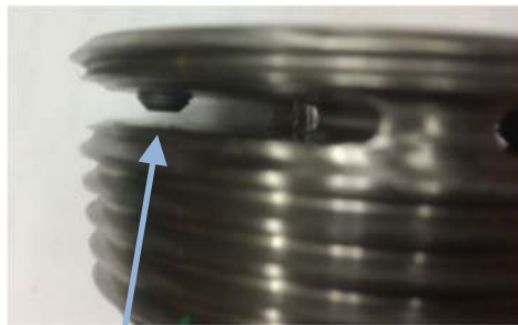
Partially Loose Set screw
