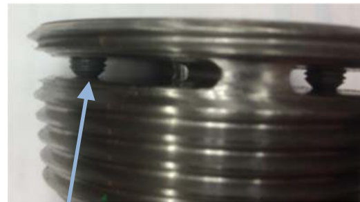
Pressed against Opposite Surface. No Gap.
