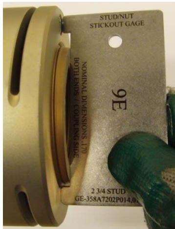
Picture 6C – Use of Stick-Out Gage
