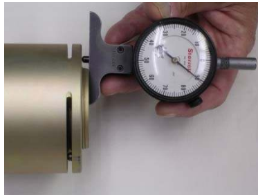
Picture 6C – Use of Drop Gage to measure stick-out
