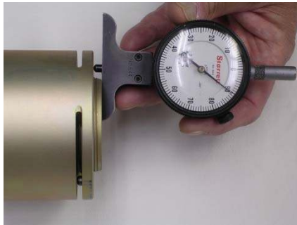
Picture 6D – Use of Drop Gage to measure stick-out
