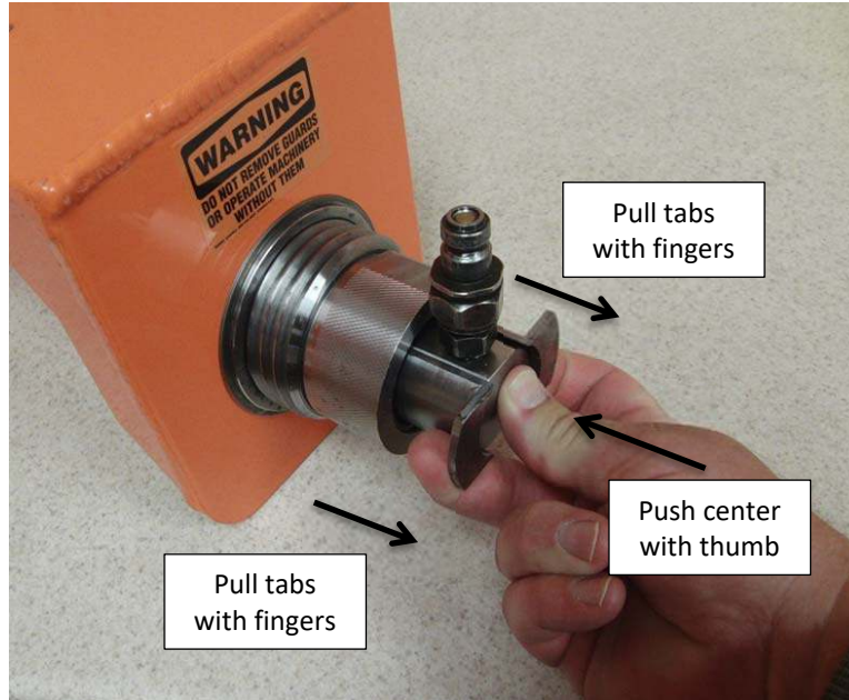
Picture 11B - Activation of the safety interlock
