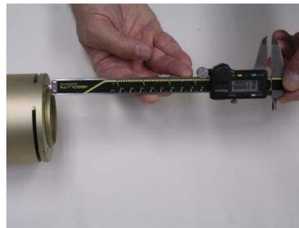
Picture 6D – Use of Calipers to measure stick-out
