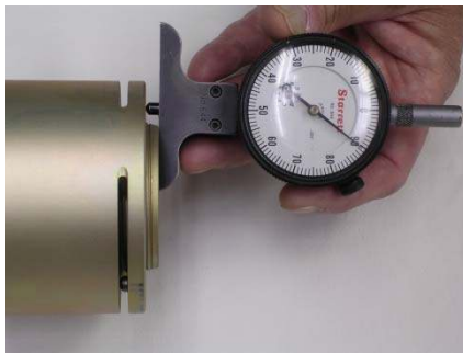
Picture 6C – Use of Drop Gage to measure stick-out
