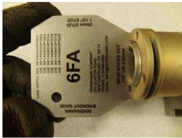
Picture 6C – Use of Stick-Out Gage on the 6FA Load Coupling stud
