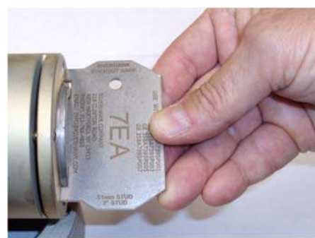
Picture 6G – Use of Stick-Out Gage on the 7EA stud
