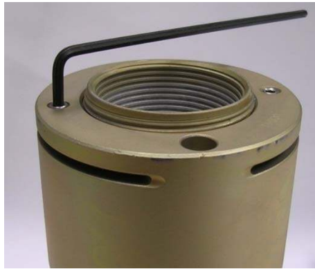
Picture 11A - Loosening of a nut's set screws
