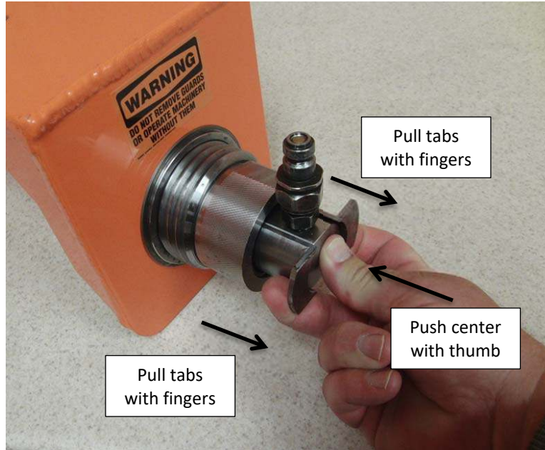
Picture 8E - Activation of the safety interlock
