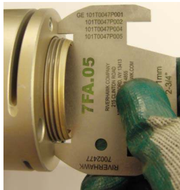
Picture 6C – Use of Stick-Out Gage on the Gas Turbine side of the Flange Joint
