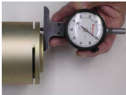
Picture 6D – Use of Drop Gage to measure stick-out
