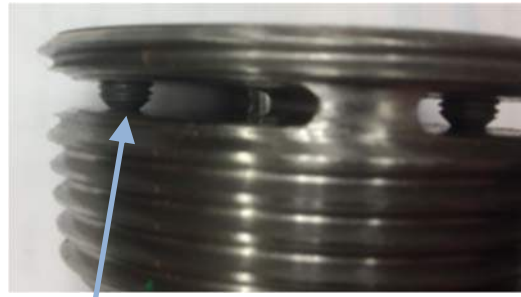
Pressed against Opposite Surface. No Gap.
