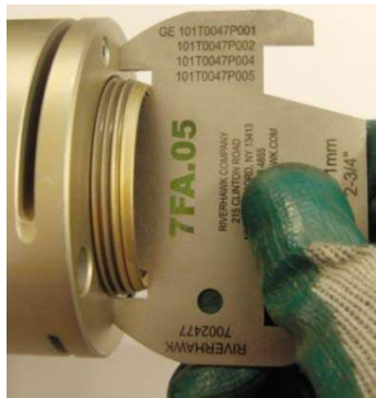
Picture 6D – Use of Stick-Out Gage on the Gas Turbine side of the Flange Joint
