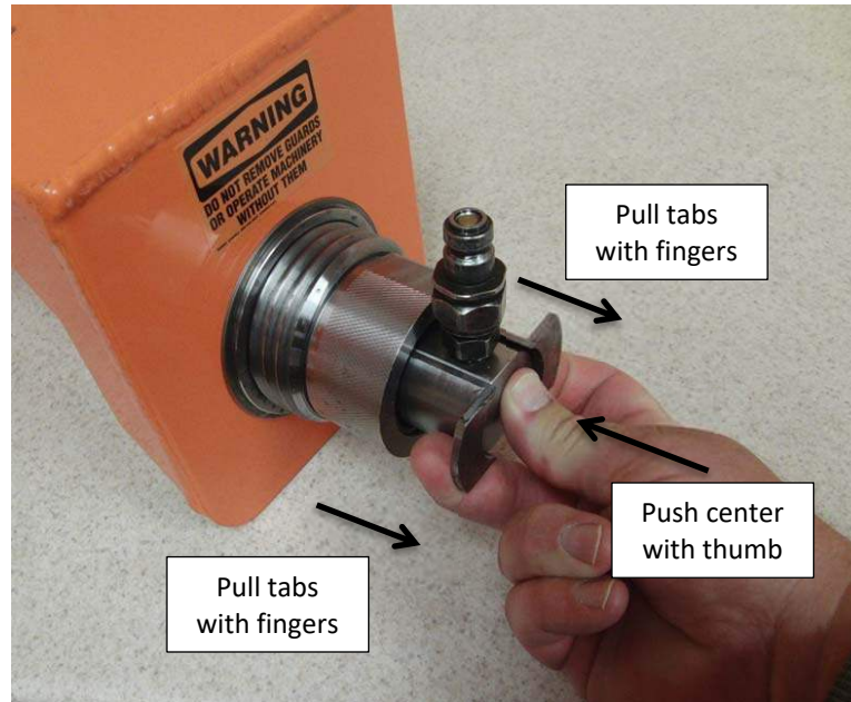
Picture 8E - Activation of the safety interlock
