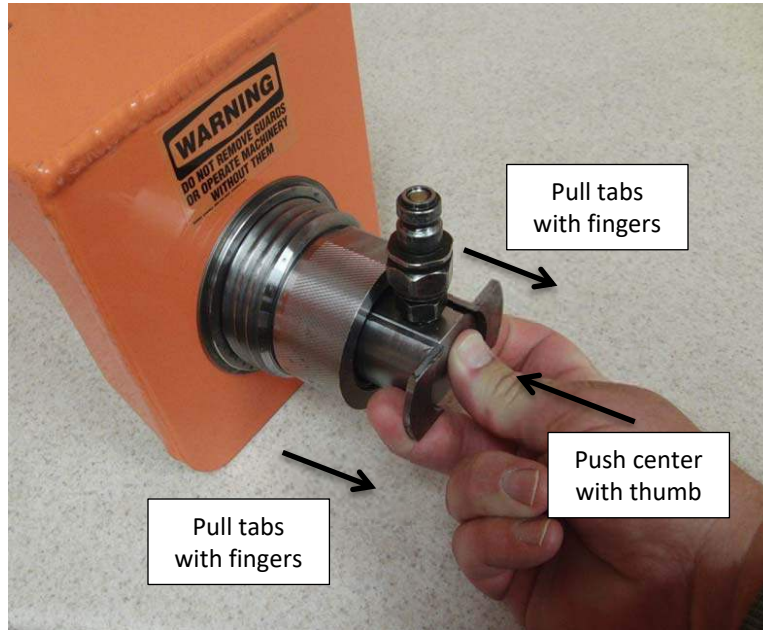
Picture 11B - Activation of the safety interlock
