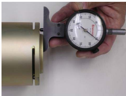
Picture 6E – Use of Drop Gage to measure stick-out
