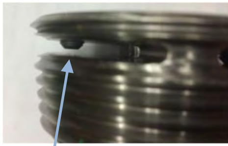
Partially Loose Set screw
