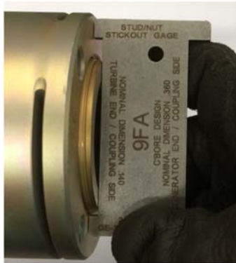
Picture 6C –How to use the Stick-Out Gage to position the stud correctly on the Gas Turbine/Load Coupling bolted flange. The gage is only used on the Load Coupling side of the flange. Use the side of the gage labeled “Turbine End/Coupling Side”.
