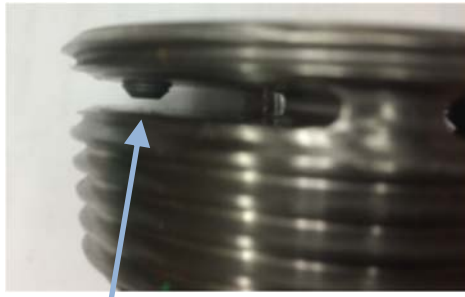
Partially Loose Set screw
