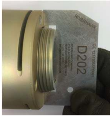
Picture 6B – Use of Stick-Out Gage on the D602 HPIP-LP Flange Joint
