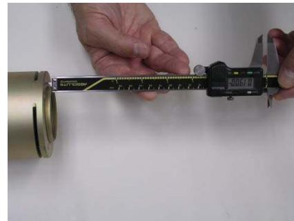
Picture 6H – Use of Calipers to measure stick-out
