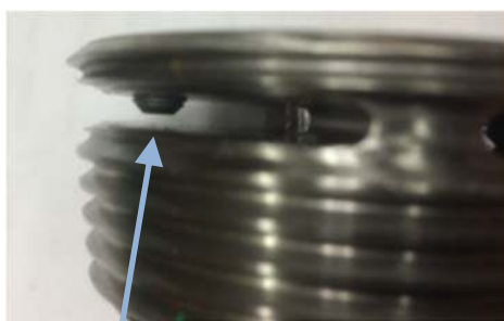
Partially Loose Set screw
