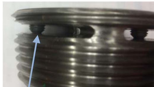
Pressed against Opposite Surface. No Gap.
