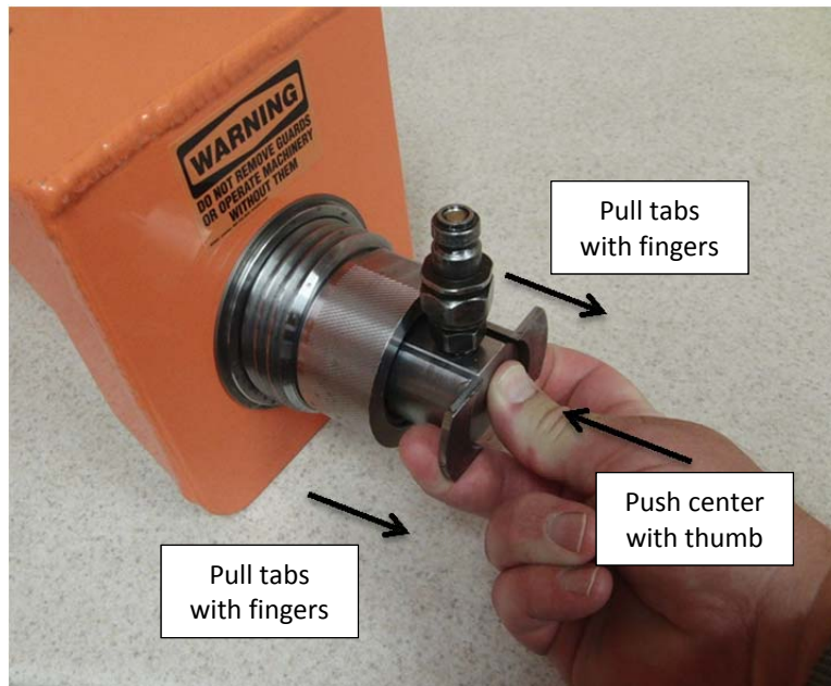
Picture 8C - Activation of the safety interlock
