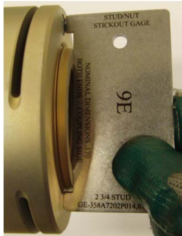
Picture 6C – Use of Stick-Out Gage
