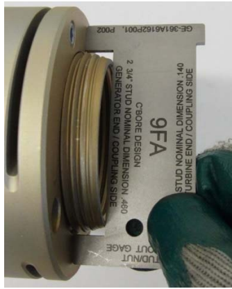
Picture 6D –How to use the Stick-Out Gage to position the stud correctly on the Load Coupling/Generator bolted flange or the Steam Turbine/Generator bolted flange. The gage is only used on the Load Coupling or Steam Turbine side of the flange. Use the side of the gage labeled “Generator End/Coupling Side”.
