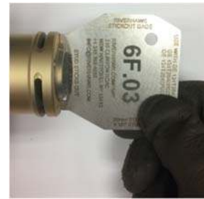
Picture 6D – Use of Stick-Out Gage on the 6F.03 Load Coupling stud
