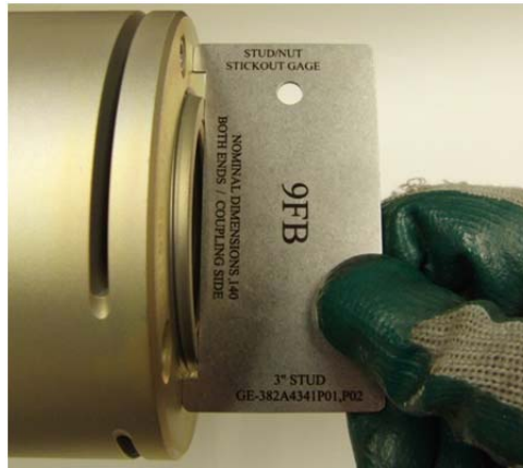
Picture 6C – Use of Stick-Out Gage
