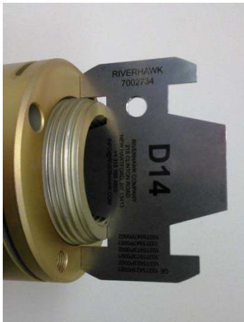
Figure 6A – Use of gage to measure stick-out
