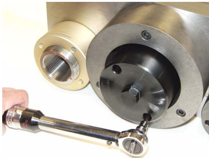
Figure 11G – Tighten screws on stud removal tool
