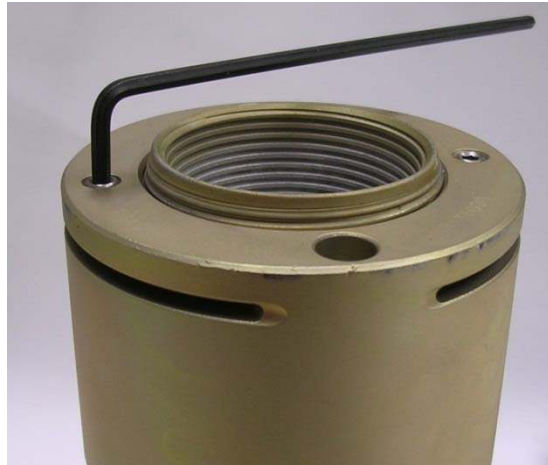
Figure 11D - Loosening of a nut's set screws
