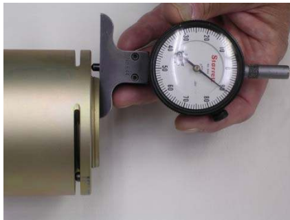
Figure 6B – Use of drop gage to measure stick-out
