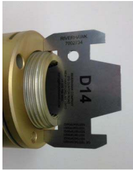
Picture 6E – D14 Gage to measure stick-out
