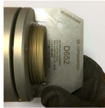
Picture 6F – D652 Gage to measure stick-out
