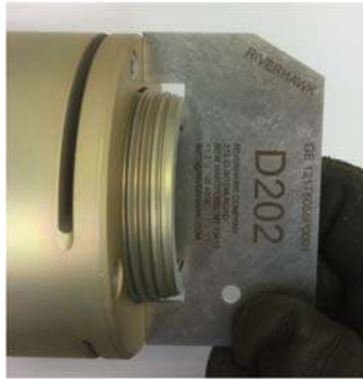
Picture 6G – D202 Gage to measure stick-out
