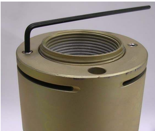
Picture 6 - Loosening of a nut's set screws
