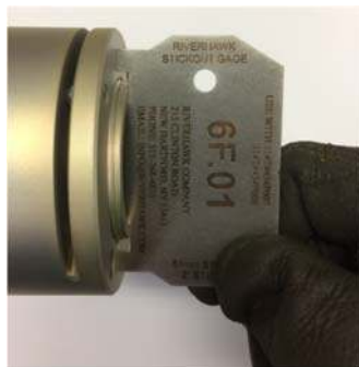
Picture 6F – Use of Stick-Out Gage on the 6F.01 Generator stud
