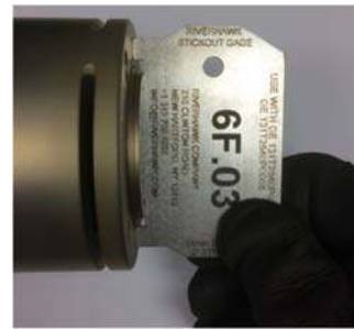
Picture 6E – Use of Stick-Out Gage on the 6F.03 Generator stud
