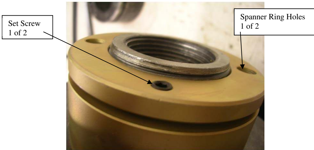
Picture 10A – Riverhawk Locknut
