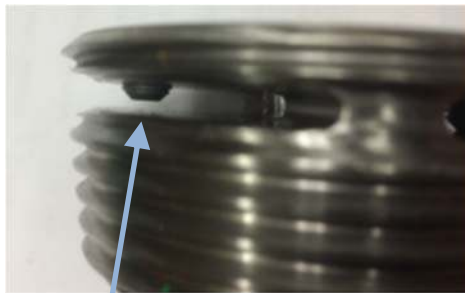
Partially Loose Set screw
