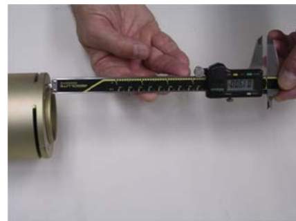
Picture 6E – Use of Calipers to measure stick-out
