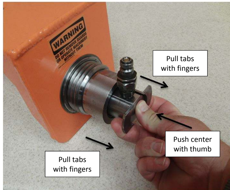
Picture 11B - Activation of the safety interlock
