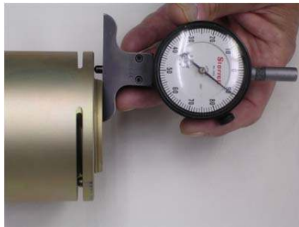
Picture 6D – Use of Drop Gauge to measure stick-out
