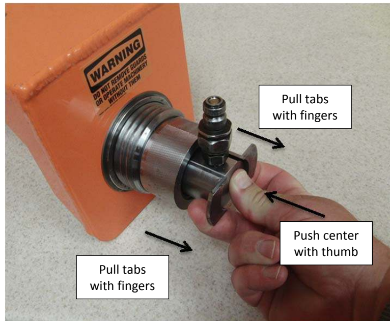
Picture 11B - Activation of the safety interlock
