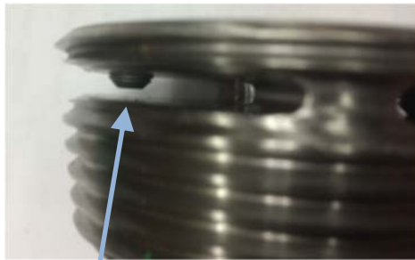
Partially Loose Set screw
