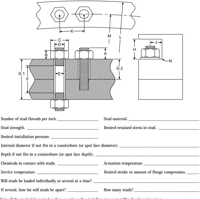
Note: If the stud stick out is less than one times the stud diameter contact Riverhawk engineering.
