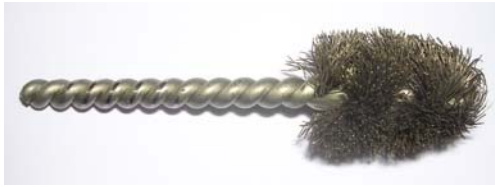
Picture of a worn brush Replace now. Do not use.
