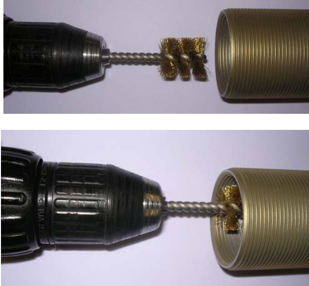
Pictures of brush cleaning of a stud
