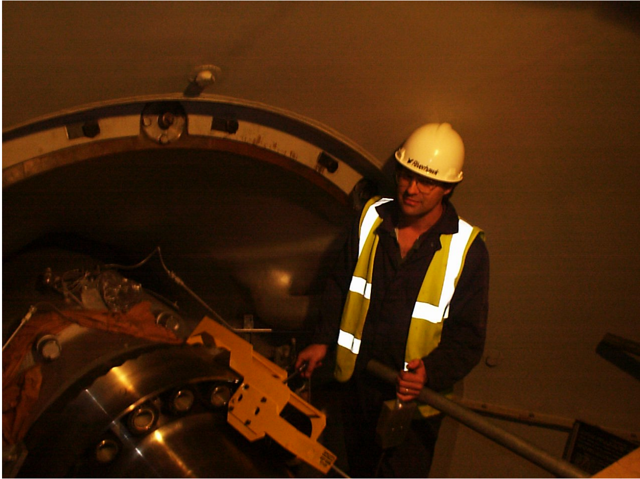
Photo 5 Tensioner during operation. Note pin wrench and control handle of pressure kit.
