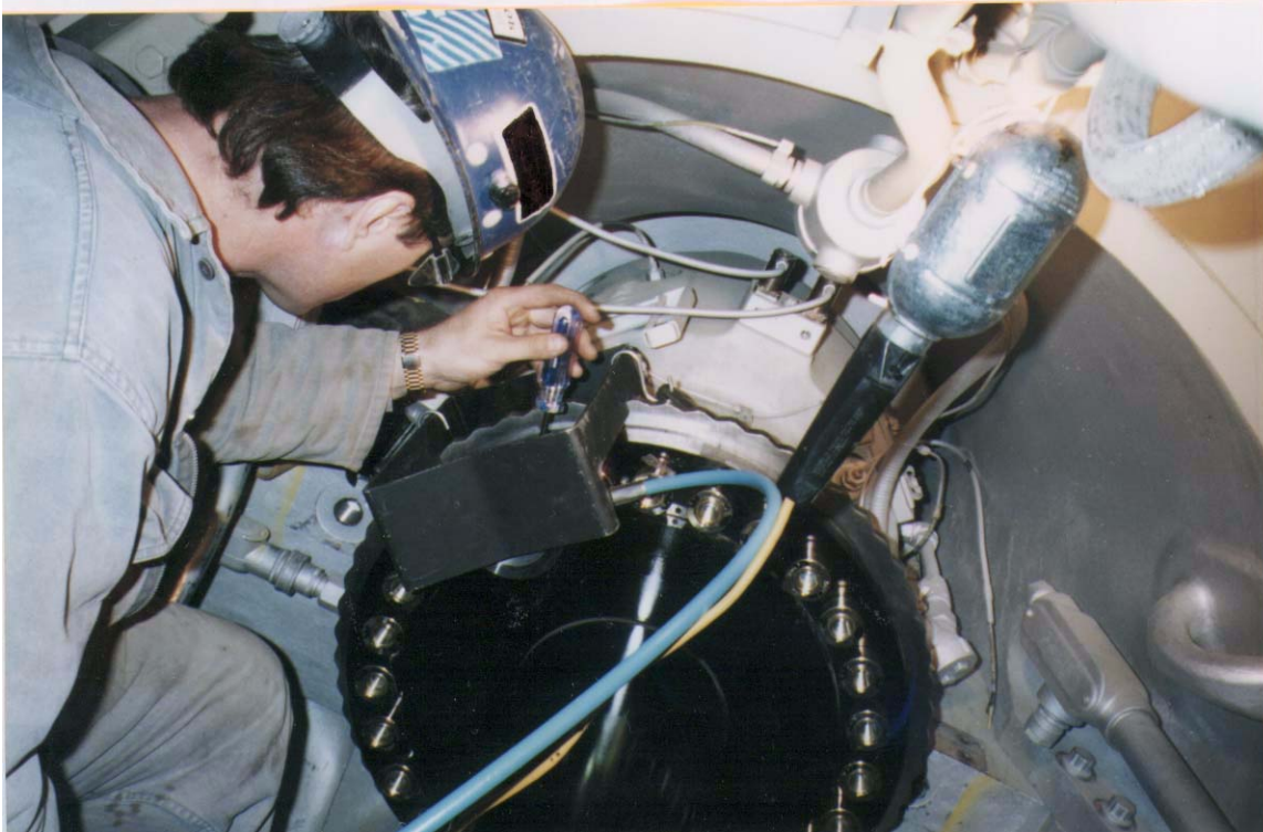
Photo 3 Top view of 1-1/8" puller tool and safety cage in place. Tool is mounted on coupling to gear flange of 6FA machine.
