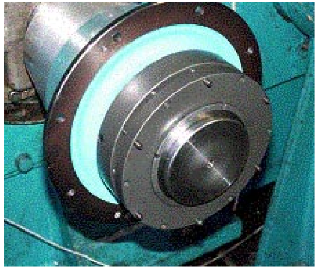
Figure 2 - Hydraulic torque coupler mounted on high speed gear.
